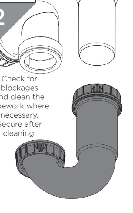
Check for blockages and clean the pipework where necessary. Secure after cleaning.
