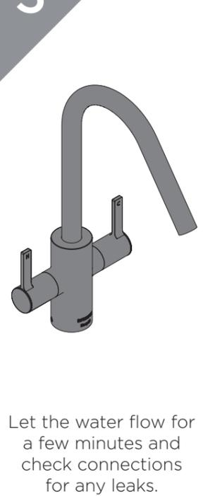
Let the water flow for a few minutes and check connections for any leaks.
