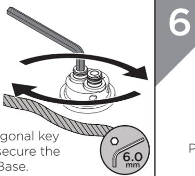
Turn the hexagonal key clockwise to secure the EasyFit Base.
