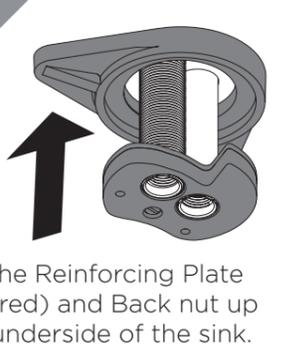
Feed the Reinforcing Plate (if required) and Back nut up to the underside of the sink.
