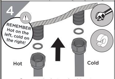
Connect the hot and cold water supplies to the threaded tails, ensuring the washers are in place.
