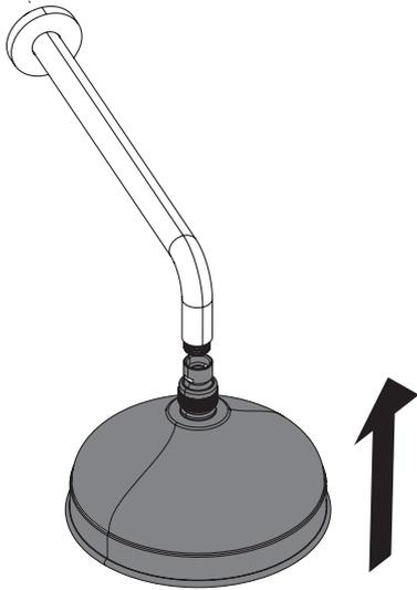
If replacing a shower rose, simply unscrew the current one and fit the new rose.
