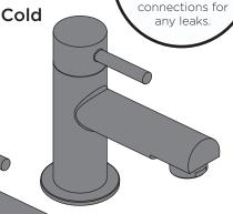
Connect the hot and cold water supplies to the threaded tails.
