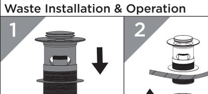
Fit the waste above the basin ensuring the washer is in place.
