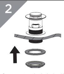
Secure waste under the basin with backnut and bottom washer
